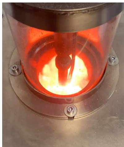
Figure 2: Pilot-scale ETFB reactor design (left) and fluidization tests in the reactor prototype (right).
